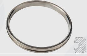
The gasket is specially used for NORSOK standard compact flange, which is mostly used for petroleum, petrochemical and offshore platforms. The special section design ensures good sealing performance under high bolt stress.
