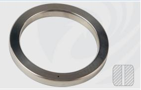
The gasket section is square, with bevels on four sides and a pressure balance hole in the middle. After the gasket is correctly installed, the flange is allowed to face to face without pressure contact. This gasket is designed to seal systems with pressures up to 20000 Psi.
