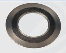
Consists of sealing element and inner and outer rings. The sealing element is confined within the inner and outer rings to prevent deformation of the sealing element. The inner ring also acts as a physical barrier against heat from the media. The outer ring ensure that the gasket is installed in the center of the flange. This gasket is suitable for raised and full face flanges in moderate to heavy service conditions.
