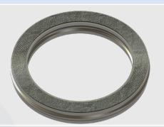
Winded by pre-formed metal strip and sealing strip, with additional winding strip at the beginning and end, which improves the strength and sealing performance. This gasket is suitable for male and female flanges, tongue and groove flanges.
