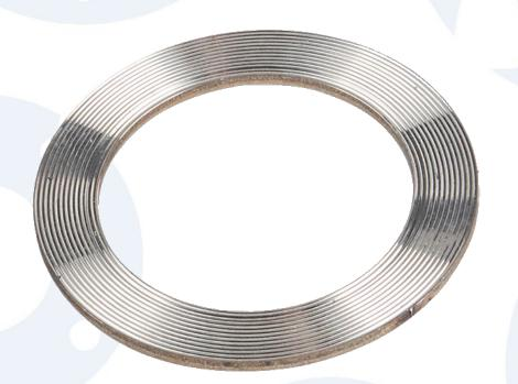
Kammprofile Gasket is comprised of a serrated solid metal core, and a soft sealing material bonded to each face. Metal core provides rigidity and blowout resistance. Sealing material provides low stress gasketing seating.
