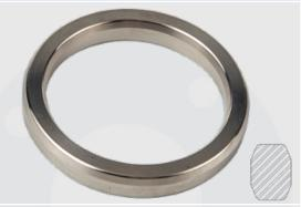
which is based on the four bevels of the gasket contacting with the flange groove to achieve the sealing effect. Applicable to flanges with flat bottom groove. Compared with elliptical ring gasket, octagonal ring gasket has better sealing effect.
