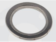
Consists of a sealing element and inner ring. The inner ring prevents sealing element from over compression and also be a physical barrier between gasket and media stream. This gasket is recommended to use for male and female flanges and tongue and groove flanges.
