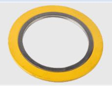
Consists of a sealing element and outer ring. The outer ring prevents over compression of the sealing element and also ensures that the gasket is installed in the center of the flange face. This gasket is suitable for raised face and full face flanges in light to moderate service conditions.
