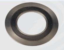
Consists of sealing element and inner and outer rings. The sealing element is confined within the inner and outer rings to prevent deformation of the sealing element. The inner ring also acts as a physical barrier against heat from the media. The outer ring ensure that the gasket is installed in the center of the flange. This gasket is suitable for raised and full face flanges in moderate to heavy service conditions.
