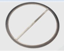
Various rib-type spiral wound gaskets can be customized according to the customer's container. Generally, it is configured with an inner ring, and winding metal strips can also be added as the outer ring. The inner ring acts as a compression stop, preventing the sealing element from being over compressed. Winding outer ring ensures that the gasket is installed in the correct position in the flange groove.
